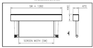
The Denham is an electrically operated roller screen. Incorporating a unique suspension system, the unit is suitable for wall, ceiling or specialized mounting. Screens up to 14.6 mtrs (48') are available.
